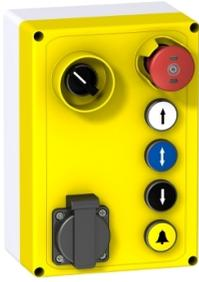
Top of car box, Harmony XALF, for lift inspection, 4 flush pushbuttons, 1 selector switch, 1 mushroom head push button, 1 mains socket
