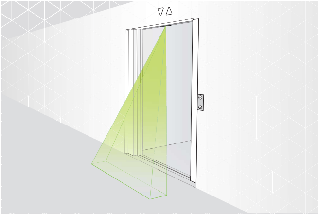
IMS 100 Pro - center-mounted for center-opening doors
