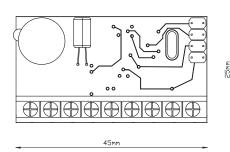
The controller **Z-5R** has a single 12V DC output for relay (included) and an iButton TM key reader input.
